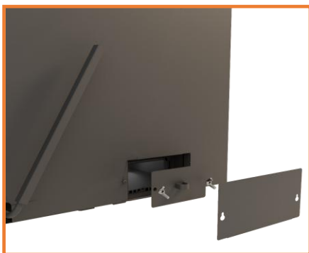
Area for cleaning ash from the boiler's rear chamber. Located at the rear of the boiler on both the left and right sides (applies to H521 and H526).
